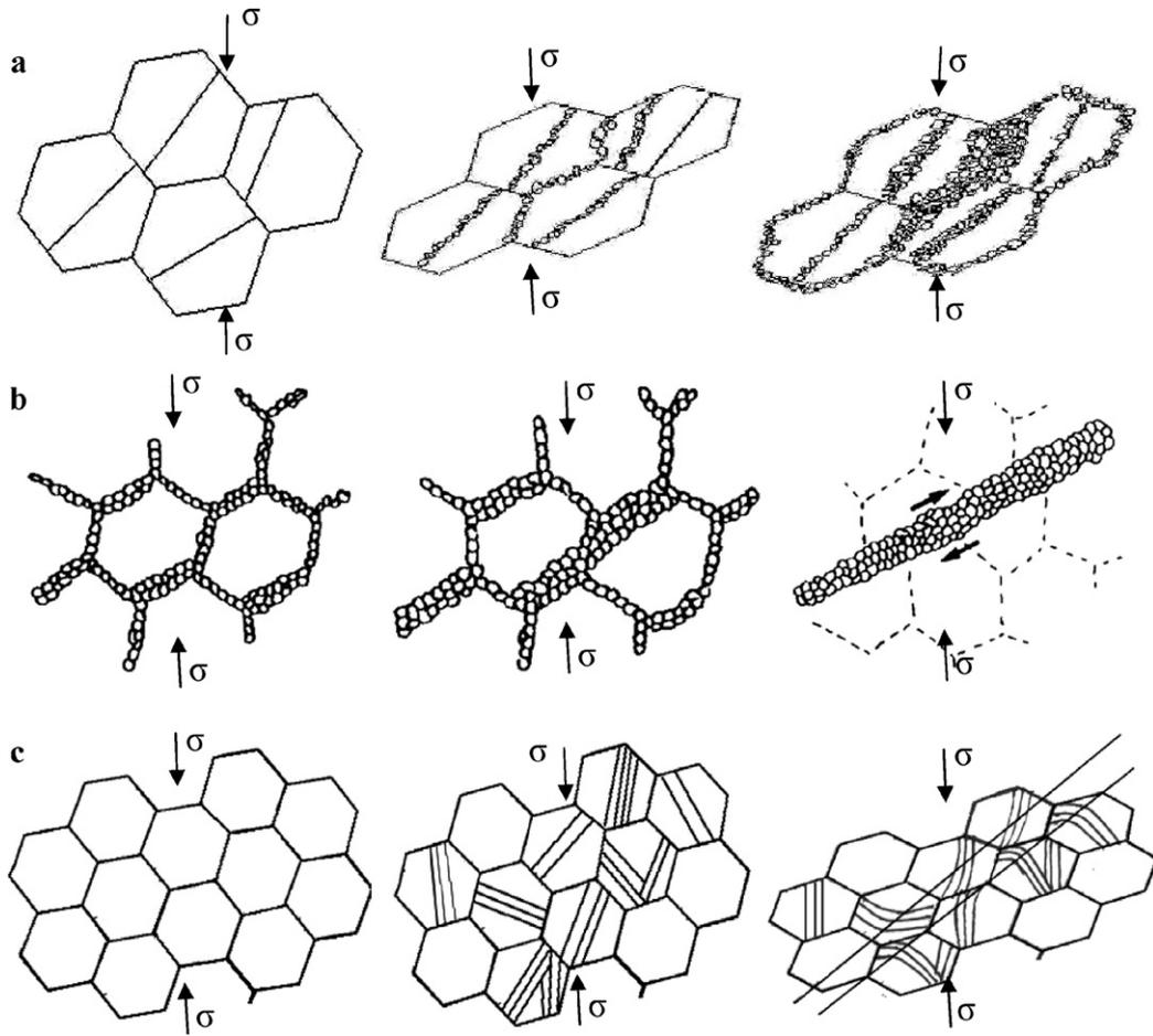
Fig. 6. Forming process of shearing bands in (a) Sample A, (b) Sample B and (c) Sample C.
