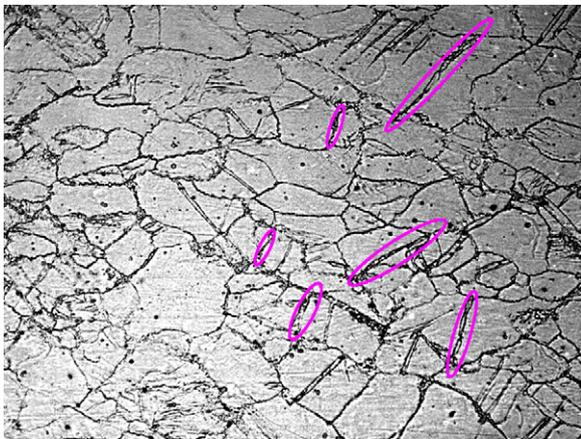
Fig. 4. The optical microstructure of Sample A after 20% rolling strain.
