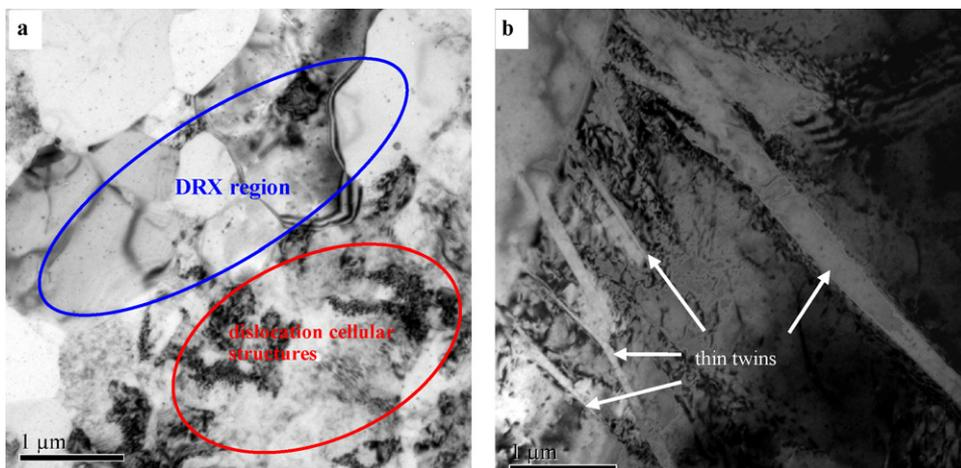
Fig. 5. (a) Dynamic recrystallized grains nucleating at original boundaries in Sample A and (b) dislocations accumulating at twinning boundaries in Sample C.
