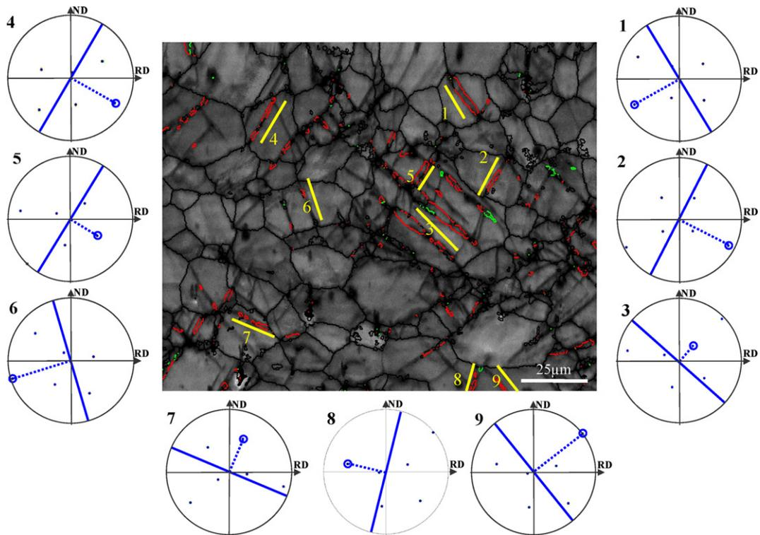
Fig. 7.  $\{10\bar{1}\}$  trace analyses in EBSD IQ map of Sample C after 20% rolling strain.
