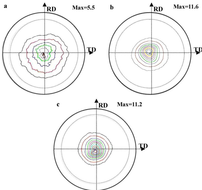
**Fig. 2.** The (0002) pole figures of (a) Sample A, (b) Sample B and (c) Sample C prior to rolling process.
