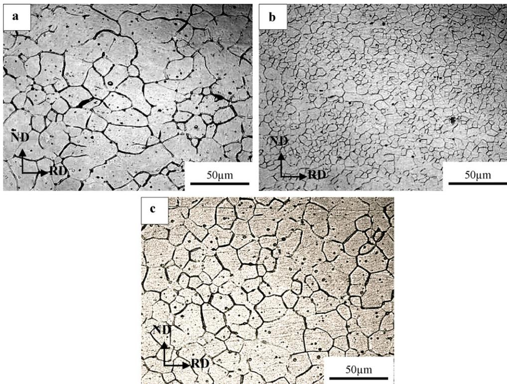
**Fig. 1.** The microstructure of (a) Sample A, (b) Sample B and (c) Sample C prior to rolling process.
