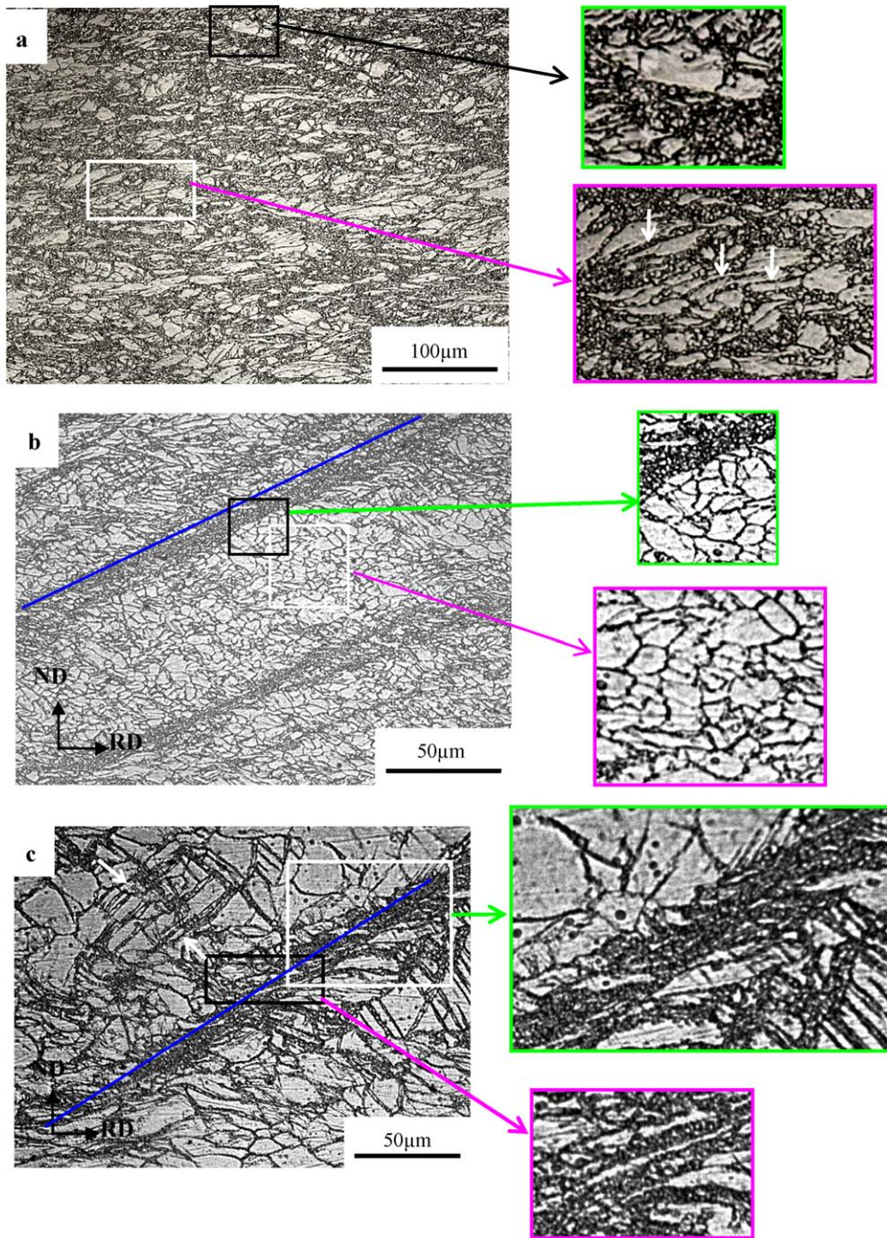
**Fig. 3.** The optical microstructure of regions close to shearing bands in (a) Sample A after 60% rolling strain and (b) Sample B, (c) Sample C after 20% rolling strain.
